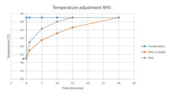
When using the sword sensor holder, pay attention to the temperature adjustment between the sword sensor holder and the sword.
