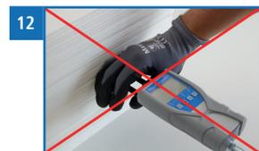
4. To ensure a correct measurement, the above mentioned pulp height must be maintained to ensure a minimum contact pressure on the electrodes.
