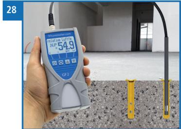
5. Now take the measured values shown on the display of the device (figure 28).
