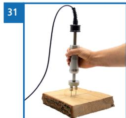
4. The device will now instantly display the moisture content on the display (figure 32).
