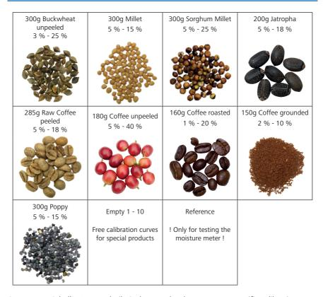
On request, Schaller Messtechnik GmbH can develop customer-specific calibration curves for special calibration curve. It is also possible to subsequently enter optionally available calibration curve into the device.
